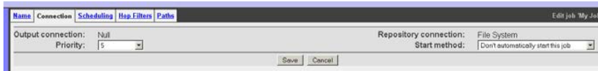
Figure 1.21: Selecting a job's connection definitions, so as to use the file system repository connection definition and the null output connection definition we created earlier.
