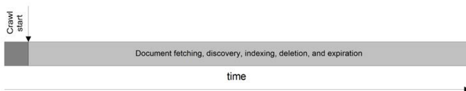
Figure 1.5: The time-based pictorial of continuous crawling shows that it doesn't really have independent phases. It continues until manually stopped.
