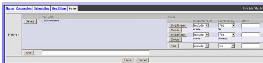
Figure 1.24: Adding a path to a file system job definition. The default rules include all files and all subdirectories.
