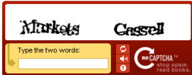
Figure 4.5 This is a reCAPTCHA widget. ReCAPTCHA allows you to load a new pair of words if you can't read the current pair, and it also provides audio CAPTCHAs for blind users.
