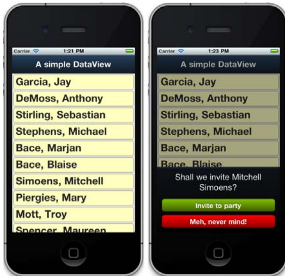
Figure 1.14 A stylized DataView with an "itemtap" event handler, displaying an action sheet based on selection.
