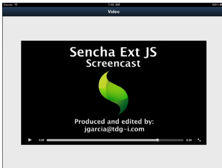
Figure 1.19 A Panel wrapping a Media widget to play video on a tablet.
