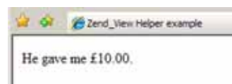
Figure 2.5 The FormatCurrency view helper is used to display the correct currency symbol in the correct place.
