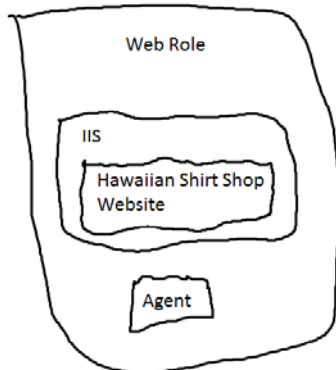
Figure 1.4 – A logical representation of the virtual machine that hosts our web application.
