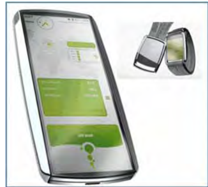
Figure 1.7 Nokia's Eco Sensor handset prototype with heart rate sensor was also designed to detect pollen levels in the atmosphere and alert allergy sufferers to this environmental hazard.
