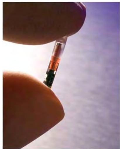
Figure 1.3 RFID chips come in all shapes and sizes, including implantable chips that can be used in the healthcare industry to diagnose disease, for example.
