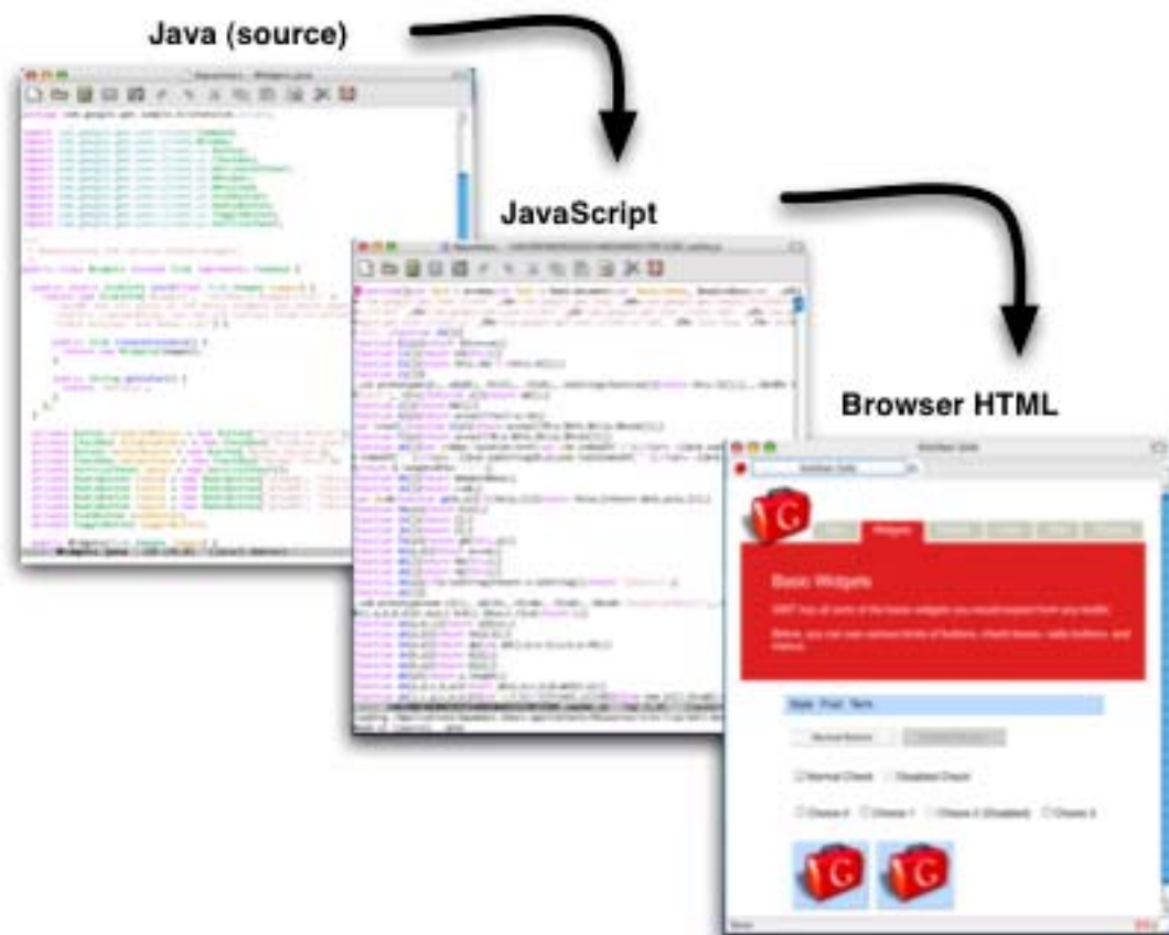
Figure 1.1 An overview of the GWT approach, Java source code that is compiled into JavaScript, which is then run in a web browser as JavaScript/HTML/CSS.
